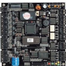
The iCON100SR is IDTECK's 13.56GHz single-door access control panel with the capacity to control up to 2 readers.
