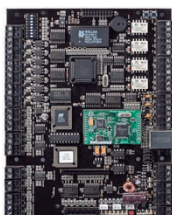
The iTDC-SR is a multi-door access control panel with the capacity to control up to 4 smart card readers.
